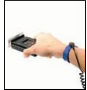
**Testing ionizer discharge time:** after charging the plate, hold the Static Sensor 718 approximately one foot (30.5 cm) away from the ionizer. Monitor the display to see how quickly the 1.1 kV charge is dissipated to 0.1 kV. The speed at which this occurs (the discharge time) indicates how well the ionizer is operating. Repeat this procedure for both a positively and a negatively charged plate.
