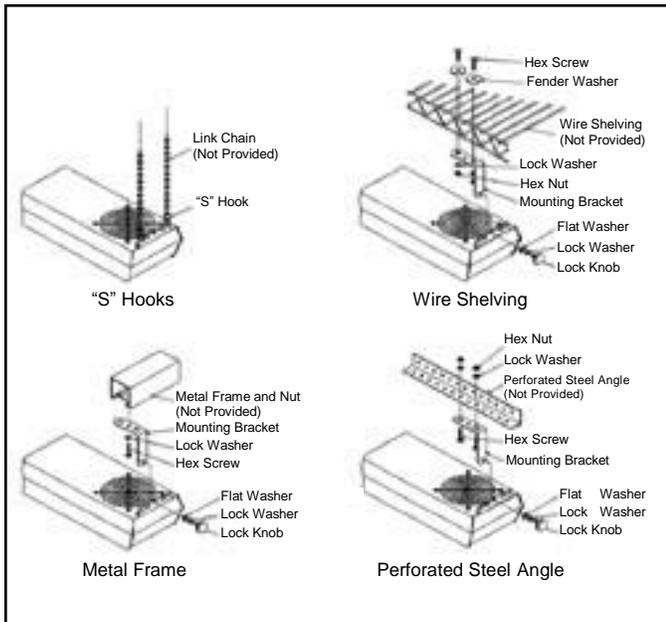
Figure 2. Mounting the SCS Overhead Air Ionizer 991A
